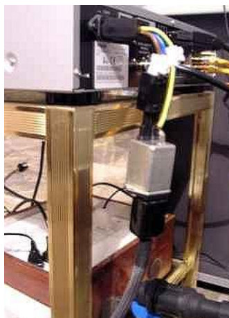
Here you can see the adapter I used to test filtered IEC mains sockets. No live parts reachable, but for your own safety please avoid replicating it.
