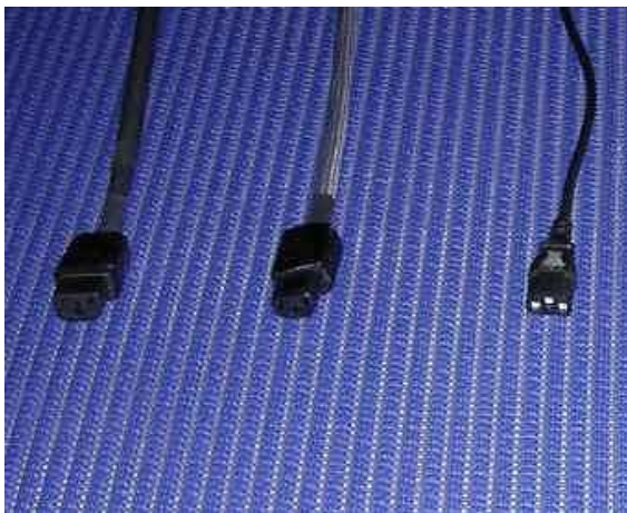
From left to right a manufacturer product – the BlackWire – and the PC Cable. First two cords have similar external diameter but quite different internal wires (3x1,5 vs. 3x2,5 – that mean 3xAWG15 vs. 3xAWG13 )
