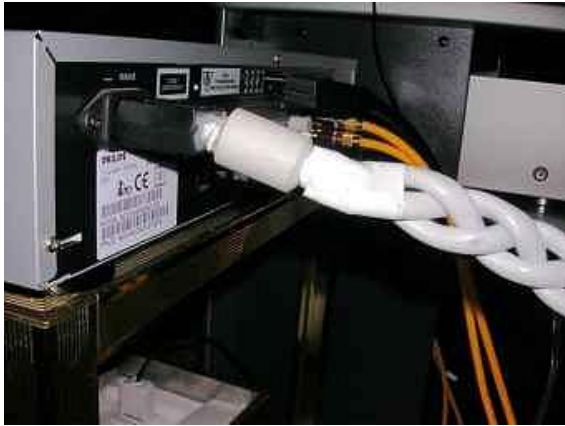
Almost straight plug in for TTS. The tape does not insulate anything, it just keep ferrite in its place. IEC cord plug is filled with silicon that, unfortunately, cannot be painted – but safety comes first.
