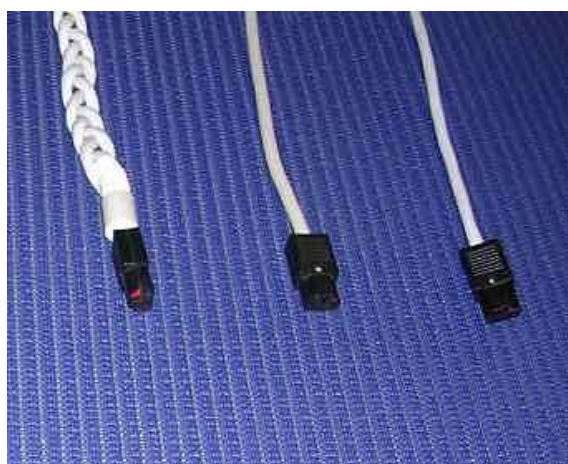
Form left to right TTS, Italian Job and SBL. An electricity phase mark on an IEC plug is not mandatory but can always be useful.
